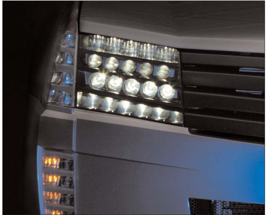
Figure 2: Visteon's LED front lighting concept
